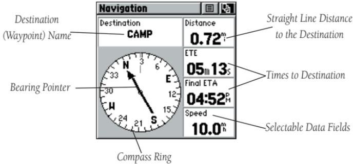
The Navigation Page provides active guidance with a rotating compass ring that shows your course over ground (track) while you're moving and a bearing pointer to indicate the current direction to your destination (bearing) relative to the course over ground.
